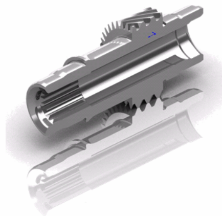
Figure 8: Inputshaft for a single speed gearbox of an electric car
